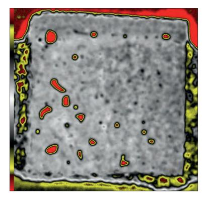
of heat swiftly, so these relatively small well-spaced voids in the die attach may pose little threat. The problem area in this component, as can be seen in Figure 1, is the right lead post and the wires attached to its top. The red areas are likely voids, but their exact placement and relative danger must be sorted out. To do so, two different imaging modes were used.
