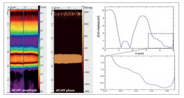
Figure 6: SCM dC/ dV amplitude and phase measurements on an *n*-type doped silicon calibration sample.
