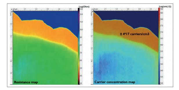
Figure 4: SSRM resistance and carrier concentration maps of an *n*-type doped silicon layer in a solar cell sample.
