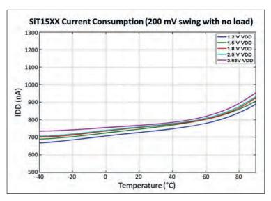
Figure 3: SiT153x draws less than  $1\mu$ A over supply and temperature.
