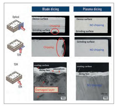
Figure 3: Damage evident on chip samples using blade dicing (left); none present when plasma dicing is used
