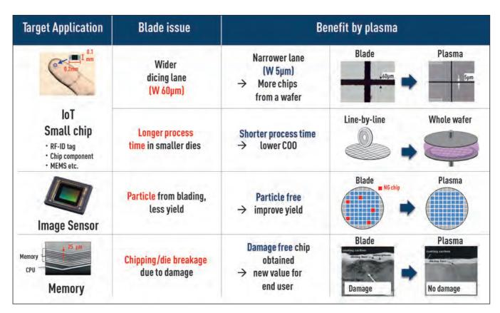
Figure 8: Benefits of Plasma in Osaka, Japan. This Class 1000 facility is capable of processing 200mm and 300mm diameter wafers with a minimum thickness of  $25\mu$ m. It is fully-equipped including two APX300 plasma dicing machines, laser pattern- ing equipment, polisher / grinder, lithography and measurement equipment, enabling customers to quickly and thoroughly evaluate different products and materials.
