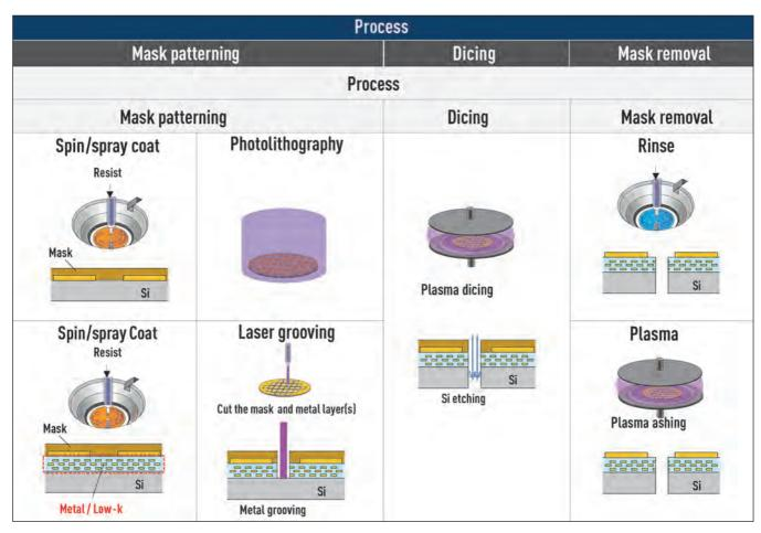
Figure 2: Panasonic's chemical etch dicing process
