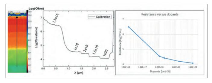
Figure 5: SSRM measurement on an *n*-type doped silicon calibration sample. The resistance cross-section is taken from the average of 50 scan lines. The resistance versus dopants data points are taken from the average resistance values measured over the 5 layers with known doping levels in the calibration sample.
