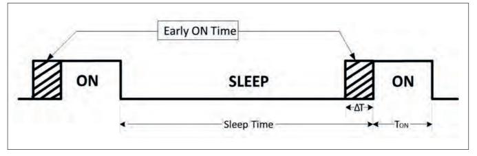
Figure 6: Early ON time (or window widening) is affected by clock accuracy and causes a power penalty.
