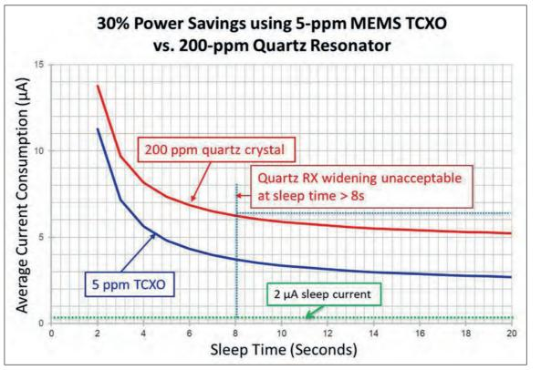
Figure 7: Power savings through use of MEMS TCXO compared to quartz XTAL resonator.
