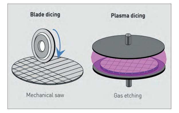
Figure 1: Blade dicing & Plasma dicing processing
