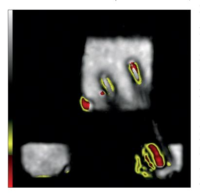
or b) if the second material is air, the pulse is almost entirely reflected, and none crosses the interface. The second possibility is useful because most of the internal structural anomalies and future field failures in a component result from cracks, delaminations, voids or other gaps containing air. A few defects that are imaged do not involve air - a tilted die, for example, or a missing solder bump, but both types of interfaces can be located and analyzed by ultrasound.
