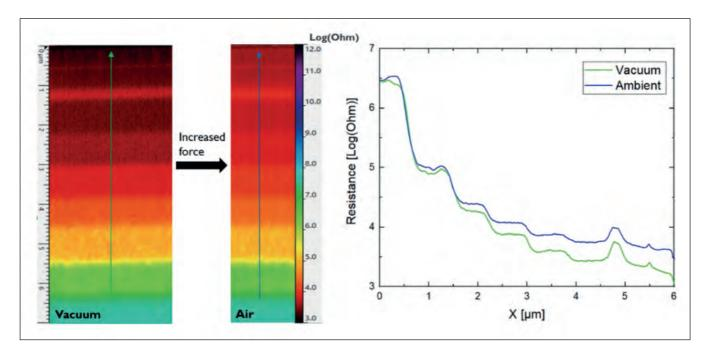
Figure 3: SSRM measurements on a *p*-type doped silicon calibration sample performed in vacuum and in air with the same probe. The resistance cross-sections are the average over 50 scan lines.
